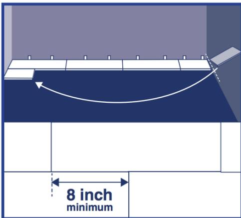
**Step 3:** Use leftover flooring from first row as starter for second row. There must be at least 20cm between flooring end joints on adjacent rows. **FOR TILE INSTALLATIONS:** The distance between end joints should be for
