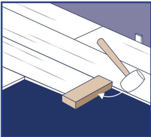
**Step 7:** Tap end of flooring with hammer and tapping block to lock ends of flooring together. Remove bridge and continue towards wall until installing the final flooring in the row.
